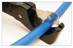
1. Cut PEX tubing square, leaving a clean, even edge. Remove any burrs.
