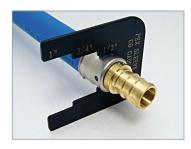
1. Slide the correct slot on the gauge around the crimped ring.
