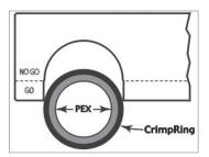
If the ring does not fit into the slot at all, then the crimp is a "No-Go". Adjust the crimping force on the tool and re-crimp the ring.
