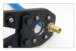
3. Set tool 1/8 in. to 1/4 in. from end of tube. Crimp sleeve with tool.
