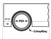
4. If the ring slides all the way into the slot, then the crimp ring is compressed too small and is a "No-Go". Remove the ring and adjust the crimping force on the tool.
