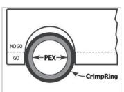
3. If the ring slides into the slot and stops in the "Go" range at least at one point, then the crimp is good. The ring will not fit the go range all the way around it.
